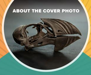
This puffin skull was made in the Denełchin Lab with a special printer that uses silica powder. The printer heats up the fine grains of silica with a laser, then binds them together, layer by layer, to create three-dimensional objects. It's like building something with sand—but the objects created by the printer are precise, strong, detailed, and resistant to heat.
